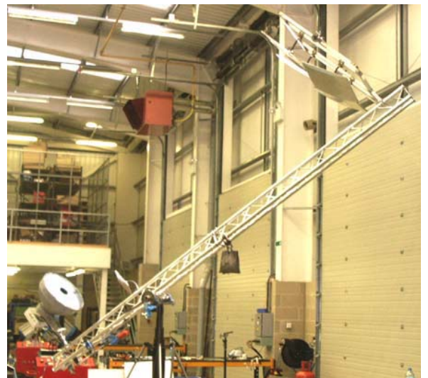
Prototype of the Lighting Crane with a little single reflector as well as with the four reflectors Main Frame
