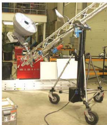
Electric elevator stand
