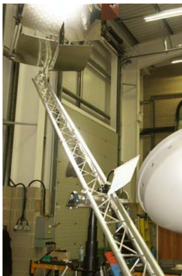
Prototype of the Lighting Crane with a little single reflector as well as with the four reflectors Main Frame
